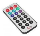
The **remote controller** provided with the kit is powered by a 3V button battery like the one shown here
